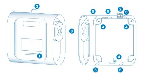
1 – LED beacon 3 – Socket-outlets\* 5 – Closing box holes
