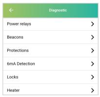
It is used to check Charge Point internal devices and diagnose possible errors. The LED beacon shows a white color during diagnostic process.
